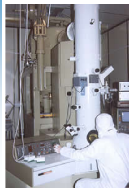
Electron beam lithography machine at IRC in Nanotechnology at University of Cambridge, England
